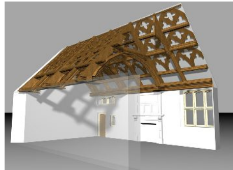
Computer image of restored hammerbeam roof.
